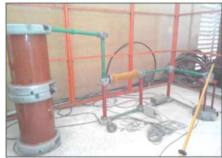
Fig.4. Dielectric strength test equipment
